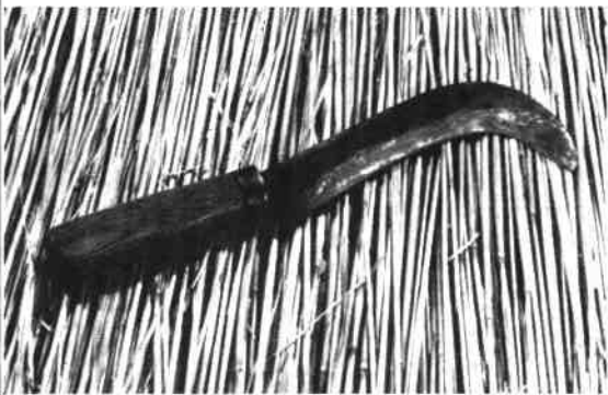
Spar-hook as used for splitting and pointing hazel spars.
