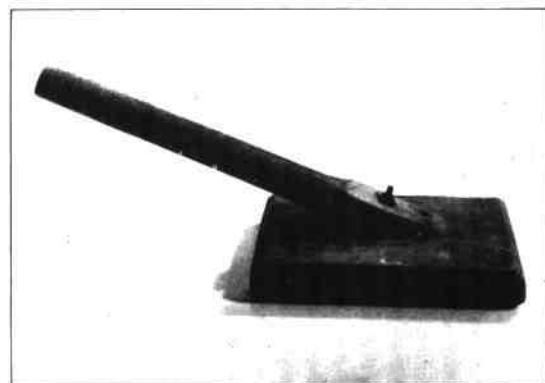
Combed wheat reed leggett of special shape as used in difficult places, e.g. between windows, valleys, etc.
