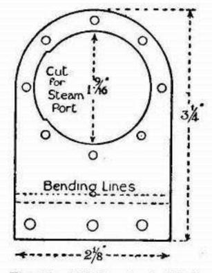
FIG. 56.—Cylinder standard before being bent.
