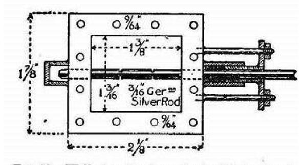
FIG. 58.—Wall-piece for steam chest, with gland and valve rod in position.
