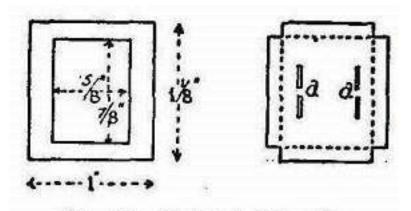
FIG. 63.-Parts of slide valve.
