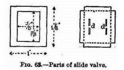
(3.) Solder the valve plate centrally to BB, and to the tops of aa, which must lie between the central and outside ports. Take great care to make steam-tight joints here, and to have the plate parallel to the standards in one direction and to the cylinder in the other. (4.) Solder in pieces *bb.* These should be a tight fit, as it is difficult to hold them in place while soldering is done.
