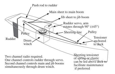
Typical method of controlling the rudder and sails of an R/C racing yacht with a two-channel radio.
