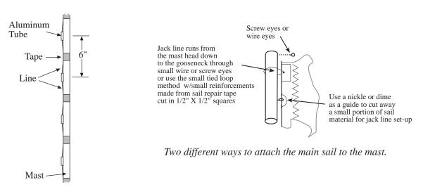
to anchor jackline ends. A drop of epoxy placed in screw hole will keep screw from working out.
