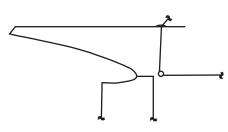
Figure 2. The mainsheet is lead to a block in the bilge of the boat, and then passed up through a small transverse slit in the deck lined with Tivar plastic.
