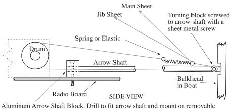
Aluminum Arrow Shaft Block. Drill to fit arrow shaft and mount on removable radio board with a couple of 4-40 machine screws.
