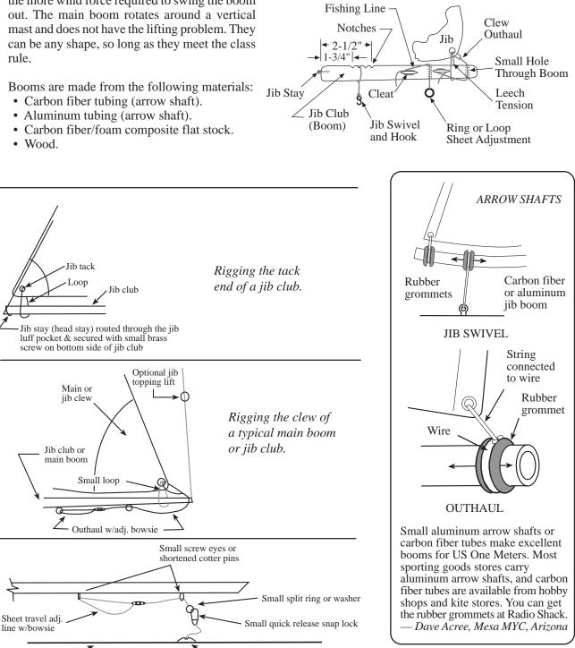
Sheet adjustment rigging for a typical main boom or jib club.
