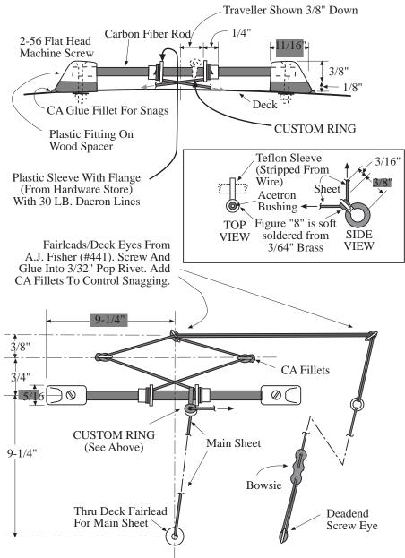
Figure 1. Main sheet traveler used by Bob Wells on his EC-12. The author believes that in winds under six to eight mph, a traveller does not make your boat go faster. However, when the wind is in the six to eight mph range or greater, a traveller increases boat speen enough to make the hassle of using it worthwhile.
