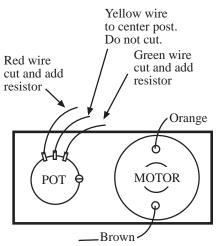
Brown and orange wires from motor to printed circuit board. DO NOT CUT.
