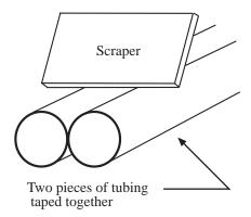
To scribe a straight line along a metal tube or aluminum arrow shaft, simply tape two identical pieces of tubing together and scribe the line with any handy piece of sheet metal with a straight edge. --Hal Robinson, Minuteman MYC, Massachusetts
