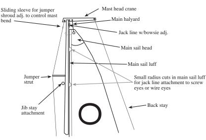
Mast head rigging of a typical fractional rig
