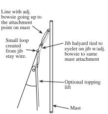
Attaching the jib to the mast on a fractional rig..
