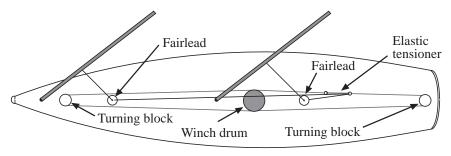
This is the sheeting arrangement used by Jim Linville for his latest US One Meter. The drum winch (a Futaba 5801) drives a loop of 80# Spectra that is lead through turning blocks at the far ends of the hull and held in tension by an elastic stretched between two rings. Sheets are fed to the booms through deck mounted fairleads. The elastic is located so that it can be replaced through the hatch.
