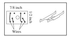
Figure 7. Layout for the new circuitboard and plastic holder to hold the trimmer pots. The author notes that a simple piece of thin plywood or plastic will also work.
