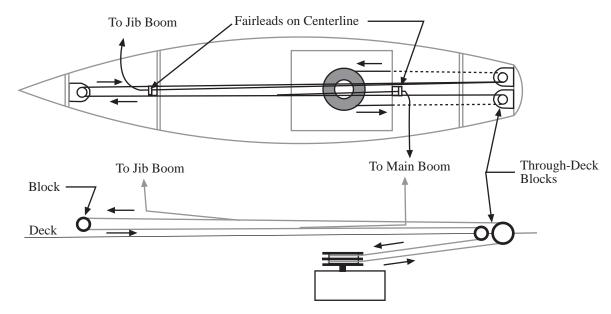
Note: The side view drawing shows the "Through Deck Blocks" as different sizes, <u>they are not</u>, they are both the same size.
