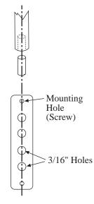
The masthead crane is made from 1/16" thick sheet aluminum, brass or fiberglass.
