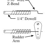
the dowel about 1" from the end. The "Z" bend or clevis should extend past the end of the dowel far enough so there is no binding, with full rudder throw. Cut the wire to length allowing for 1/4" right angle bend. Insert the 1/4" bend in the 1/16" hole in the dowel. Wrap the wire and dowel with string, then Zap it. Do both ends of dowel.
