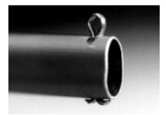
This is the end of one of Hal Robinson's booms. Hal makes them from aluminum arrow shafts that he heats with a torch until the aluminum begins to change color. He then lets them cool slowly to room temperature before bending curves to match the foot of his sails. After bending, the shaft is flattened between two boards in a vice. Hal says he has to overbend the curve because some of it will come out during the flattening procedure. Note the neat use of a cotter pin as a strap eye.
