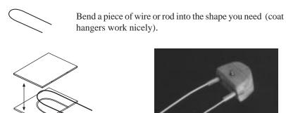
Place the wire shape between two pieces of 1/8 inch balsa and press together to form an indent in the balsa.
