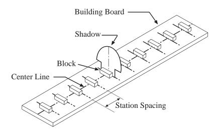
The board has to be "warp-free". It can be plywood or particle board shelving material. Particle board is a little more difficult to cut and drive nails into than plywood. Size of the board is about 5/8" x 12" x 48". If you want to keep the board clean, cover it with shelf paper.
