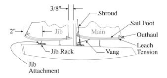
attachment back to about 2 1/2 inches. If wind is light use 1 3/4 inches. Move the attachment at boom and Jib deck rack to maintain 3/8" spacing (slot) between Jib and Mast.
