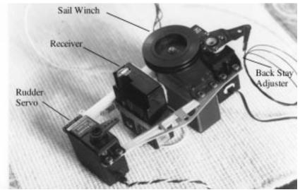
Not all redio boards are wood. This one is made from a couple of aluminum angle irons that are mounted in the hull with simple brackets hung from the centerboard trunk.
