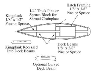
Deck beams can be flat which gives a flat deck, or curved so the deck is crowned. Deck beams should be located at the jib pivot, near the sheet exit guides and the mast.
