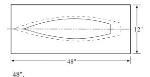
Place the hull on plywood, deck side down. Trace
