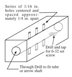
A through drilled piece of 3/4 inch square aluminum stock approximately two inches long makes a great jig for drilling arrow shafts and other tubing. Size the through hole to match the O.D. of the shaft. A 6-32 set screw lock everything in place for drilling. One person I know made one of these jigs from oak — minus the set screw, and it seems to work fine.
