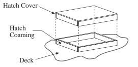
be a tight fit to prevent water from getting into the interior of hull.
