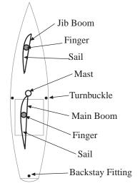
With sails let out set Jib boom approximately 2 deg. beyond right angle. Allow some slack in Main sheet. When sails are pulled in slightly the Jib will be at right
