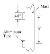
Thread tubes on a length of line (heavy fish line). Stretch line along trailing edge of mast. Secure ends of line with masking tape.
