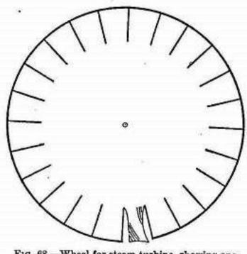
FIG. 68.—Wheel for steam turbine, showing one vane twisted into final position.
