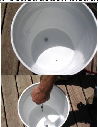
13. To the other side of the bucket bottom, drill a second 1/2inch diameter hole in the bucket marking the location on the bucket lid with the drill.
