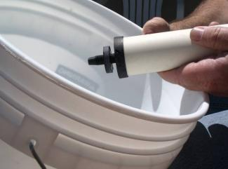
19. Gently push the filter through one of the holes drilled through bucket bottom and bucket lid.
