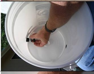
8. Using pliers tighten the spigot to the bucket with a nut. This with have to be a very tight fit to create a water tight joint.
