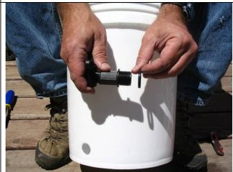
6. Push the spigot with washer attached through the hole drilled in Step 3.
