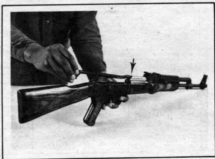
FIGURE 43. REPLACING DRIVING SPRING
