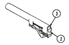
Step 4. Check for cartridge nose jamming against upper chamber (3).
