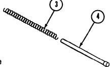
Step 4. Check to see if the recoil spring (3) and spring guide (4) are damaged or broken.
