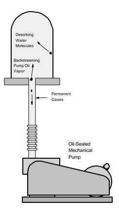
Figure 1 - Residual Gases at Base Pressure
