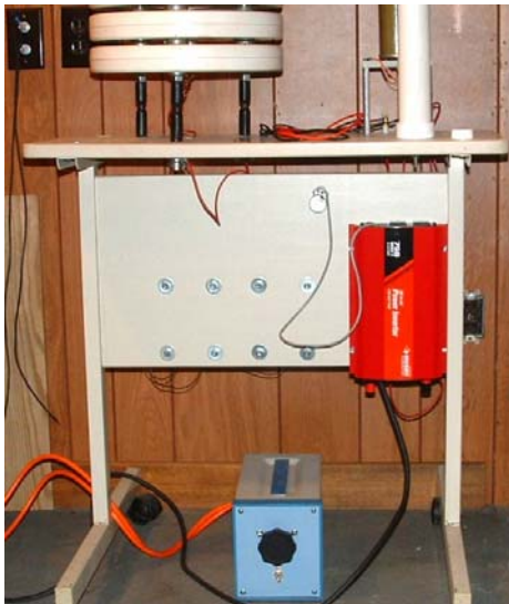
Figure 6 - Power Supply with Vector 750 Watt Inverter. The 400 Hz autotransformer is in the box on the floor. In operation this would be remote from the stand. The frequency adjustment pot is above and to the left of the inverter.
