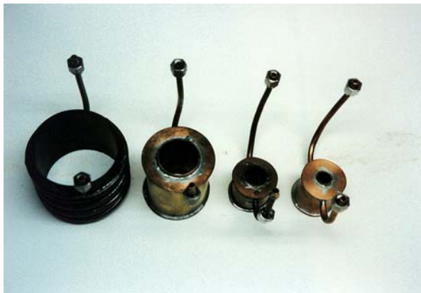
Figure 6 - Various cooling coils. At the left is the original 3" id coil.
