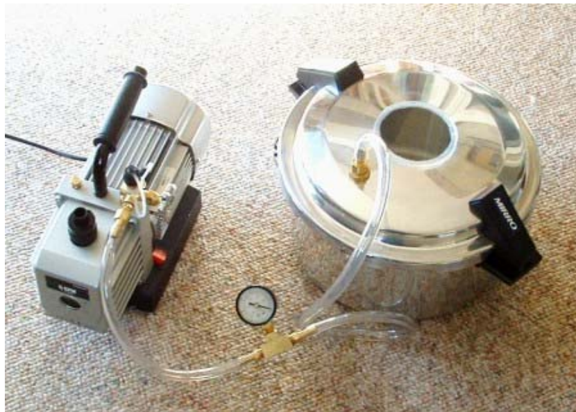
Figure 3 - Gel Candle Deairing Apparatus with Metal Chamber
