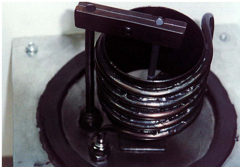
Figure 3 - Upper graphite rod and cooling coil in place.
