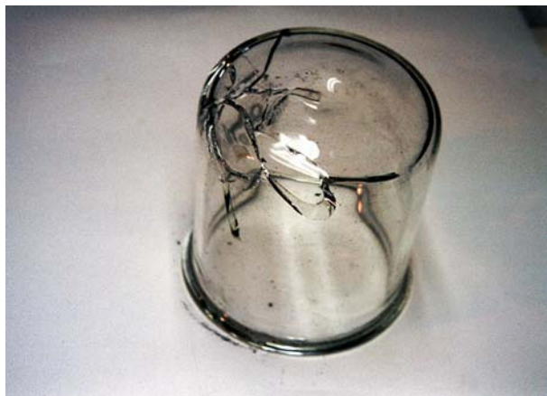
Figure 1 - Fractured Bell Jar
