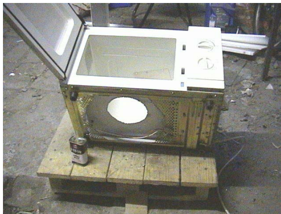
Figure 4 - Oven with hole cut into bottom of cavity.
