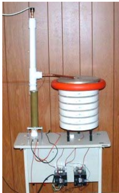
Figure 2 - The author's conversion with six-section 120 kV negative cascade, dual 10 kV rms transformers, water resistor and 1 Gohm divider resistor.
