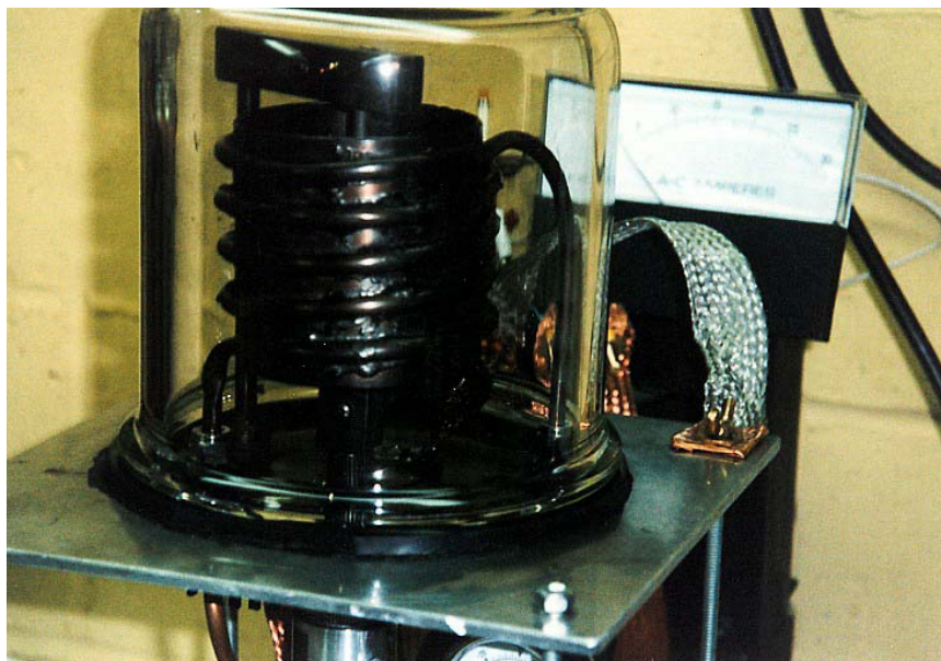
Figure 4 - Assembled reactor without the safety shield.
