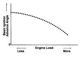
There are other sensor inputs which also affect the basic spark advance angle. The A/C compressor clutch signal advances basic spark angle when the IDL contacts are on (on some engines), and on the 3S-GTE engine, basic advance angle is retarded if the ECU judges that regular fuel is being used, based on signals from the engine knock (KNK) sensor.
