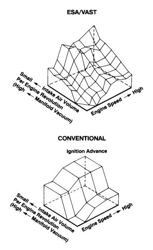
To provide for optimum spark advance under a wide variety of engine operating conditions, a spark advance map is developed and stored in a look up table in the ECU. This map provides for accurate spark timing during any combination of engine speed, load, coolant temperature, and throttle position while using feedback from a knock sensor to adjust for variations in fuel octane.
