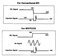
As the IDL contact opens, the ECU commands all injectors to simultaneously deliver an extra asynchronous injection pulse.
