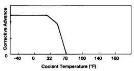
As the engine temperature approaches overtemp, the ECU will advance spark when the IDL contact is on, to prevent overheating. When the IDL contact is off, the ECU will retard spark to prevent detonation. Advance and retard shown on the graph are corrections to the basic advance angle.
