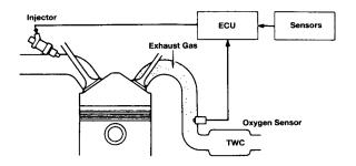
By achieving more accurate fuel metering, the oxygen content of the exhaust stream is held within a very narrow range which supports the most efficient operation of the three-way catalyst (TWC).
