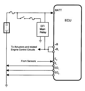
The ECU cannot properly function without dependable power feeds and ground circuits. The power distribution system involves several electrical circuits, protection devices, relays, and grounds.
