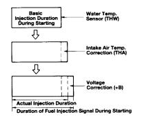
Injection duration while cranking is corrected for battery voltage by increasing injection duration at lower voltage.
