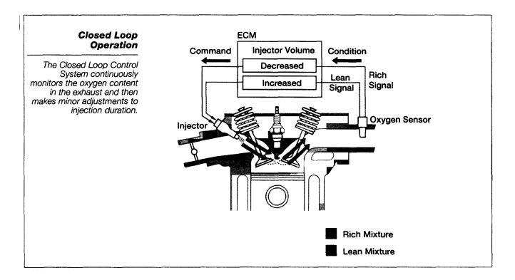
Closed loop control works on the premise of the command changing the condition and can be summarized as follows:
