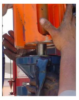
Insertion of motor spline into the pump keyway. Cut away of a small submersible pump.
