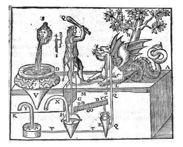
When the human figure is turned toward the dragon, a valve between the two sealed chambers under the figure closes. However if the human figure is rotated to the side, the valve connecting the two chambers opens, water flows from the top to the bottom chamber, and suction is created in the pipe leading from the upper chamber to the dragon's mouth. Because of this suction, the dragon appears to drink if a cup of water is held up to its mouth. (Buch von Lufft-Und Wasser-Kunsten, page 3)
