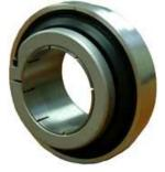
You should replace a mechanical seal whenever the seal is removed from the shaft for any reason, or whenever leakage causes undesirable effects on equipment or surrounding spaces. Do not touch a new seal on the sealing face because body acid and grease or dirt will cause the seal to pit prematurely and leak.
