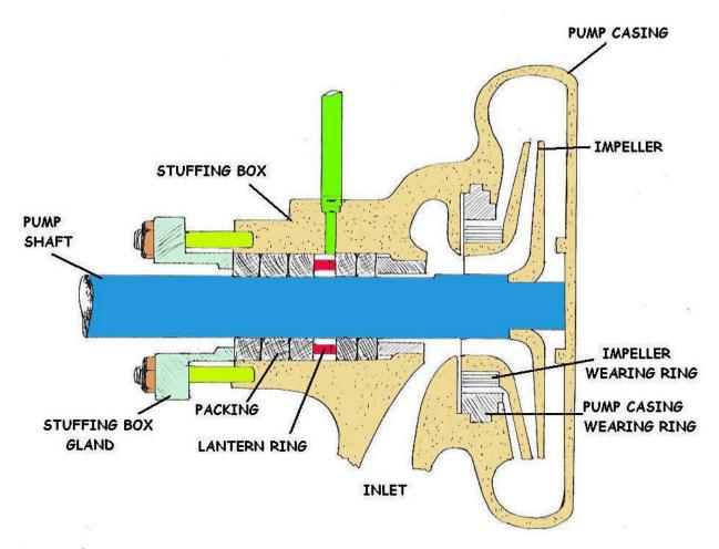
A centrifugal pump has two main components:
