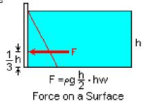
obtained from the integral of  $dM' = \rho gxy \, dA$ , the moment about some vertical line in the plane of the surface. If there happens to be a pressure on the free surface of the water, then the forces due to this pressure can be evaluated separately and added to this result. We must add a force equal to the area of the surface times the additional pressure, and a moment equal to the product of this force and the distance to the centroid of the surface.
