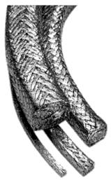
absolutely necessary to use the correct packing. When replacing packing, be sure the packing fits uniformly around the stuffing box. If you have to flatten the packing with a hammer to make it fit, **YOU ARE NOT USING THE RIGHT SIZE.** Pack the box loosely, and set up the packing gland lightly. Allow a liberal leak-off for stuffing boxes that operate above atmospheric pressure.
