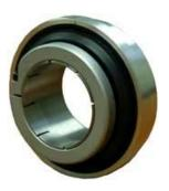
You should replace a mechanical seal whenever the seal is removed from the shaft for any reason, or whenever leakage causes undesirable effects on equipment or surrounding spaces. Do not touch a new seal on the sealing face because body acid and grease or dirt will cause the seal to pit prematurely and leak.
