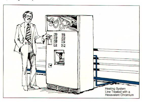
Several cross-connection have been made to soda machines, the one to worry about is when you have a copper water line hooked to  $CO_2$  without a backflow preventer. The reason is that the  $CO_2$  will mix in the water and create copper carbonic acid, which can be deadly. This is one reason that you will see clear plastic lines at most soda machines and no copper lines. Most codes require a stainless steel RP backflow assembly at soda machines.
