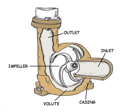
These pictures illustrate the components that are common to most pump assemblies.
