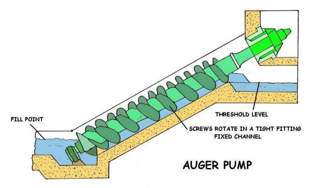
The machine consists of a screw inside a hollow pipe. Some attribute its invention to Archimedes in the 3rd century BC, while others attribute it to Nebuchadnezzar II in the 7th century BC. A screw can be thought of as an inclined plane (another simple machine) wrapped around a cylinder.
