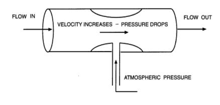
The newest injector design causes complete mixing of injected materials (air, ozone or chemicals), eliminating the need for other in-line mixers. Venturi injectors have no moving parts and are maintenance free. They operate effectively over a wide range of pressures (from 1 to 250 psi) and require only a minimum pressure difference to initiate the vacuum at the suction part. Venturis are often built in thermoplastics (PVC, PE, PVDF), stainless steel or other metals.
