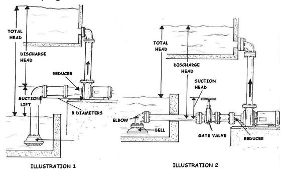
Here are the important points to consider about suction piping when the liquid being pumped is below the level of the pump:
