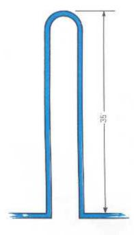
The barometric loop consists of a continuous section of supply piping that abruptly rises to a height of approximately 35 feet and then returns back down to the originating level. It is a loop in the piping system that effectively protects against backsiphonage. It may not be used to protect against back-pressure.
