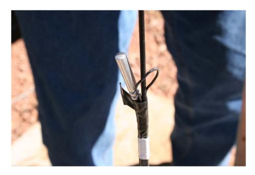
Blasting cap on the explosive cord. Below, some of the debris from inside the well casing following the explosion. After talking to this man, I found out that after 9-11, he had to increase his fees because of the ATF and new rules concerning explosives. Be prepared to pay through the nose for this treatment process. Consider this expense the price of admission to having adequate water to supply your customer's demands.
