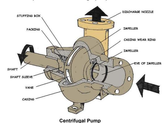
As the impeller rotates, it sucks the liquid into the center of the pump and throws it out under pressure through the outlet. The casing that houses the impeller is referred to as the volute, the impeller fits on the shaft inside. The volute has an inlet and outlet that carries the water as shown above.
