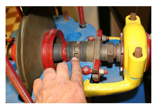
Finger is shown pointing to a Lantern Ring. This old school method of sealing a pump is still out there. Notice the packing on both sides of the ring. The packing joints need to be staggered and the purpose of this device is to allow air to the Stuffing Box.
