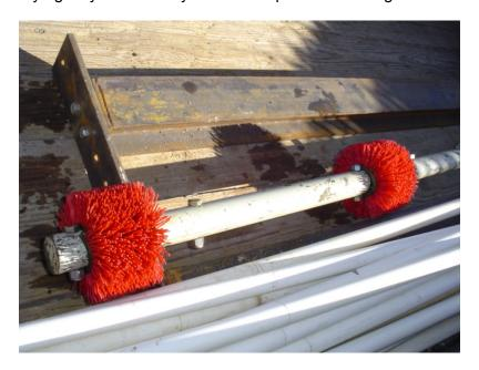
This brush is used to dislodge debris inside well casing. Just a big toilet cleaning brush.
