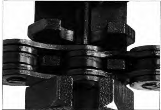
Breaking and joining a chain is easy once you have the 'knack': begin by practising on an old length of chain. First nest the chain in the chain tool with the outer link plate braced and the pin exactly centred on the rivet.
