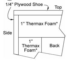
\*Thermax, Tuff-R, Celotex, R-Max, etc, foil-faced urethane (polyisocyanurate) foam
