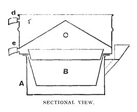
constructed specially for evaporating and distilling; it is low and shallow, having a large bottom surface, fitting it well for distillation. rapid evaporation and Fenner's Water-bath Percolator and Still may be employed for the same purposes, but as it is constructed for percolation also, corresponding sizes do not present so large a surface for evaporation and
