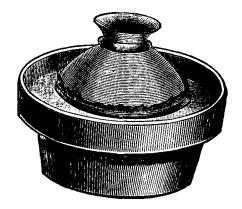
In pharmacy, dialysis is employed to separate what are known as *colloid* (gluelike) substances, from their combination in solution with crystallizable substances. This is accomplished by means of an apparatus called a Dialyzer, a simple form of which is here illustrated.
