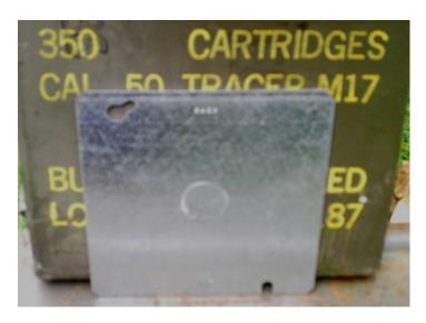
Stove doors can be improvised in many different ways. This electrical box cover plate makes a good door. Stove doors can be mounted on the stove with hinges, or they can just be wired on. Doors made from flat plates can be attached with a single bolt, so that they can pivot open. Use a simple wire handle on your door, to avoid burns.
