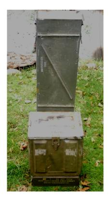
The chimney box can be bolted, screwed, wired, or welded to the stove box. The stove can sit on the bare ground, or on rocks or cinder blocks, or it can have legs made from bolts or angle iron, or it can be elevated on one or two extra ammo cans (which should be open, or at least punctured, to keep them from bursting from the intense heat).
