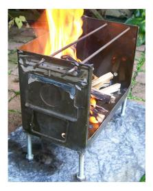
Ammo Can Fire Box: A large ammo box can be made into a good fire box, by cutting one side open with a hacksaw. Four large bolts were used to make legs for this fire box, but it could have been set on bricks, or cinder blocks. The metal rods are intended to support cooking pots, but any type of expanded metal screen would work, and would also allow grilling.
