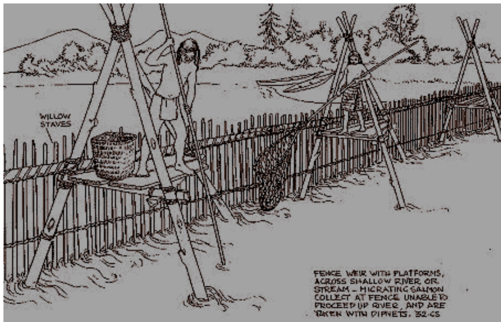
Fence Weir: The fence weir is a fence built across a stream, to block fish moving upstream. Fish milling along the fence line are either speared, or collected in dip nets, from platforms.
