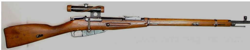
The Mosin Nagant M91/30, a bolt-action 30 caliber rifle in 7.62 x 54R.
