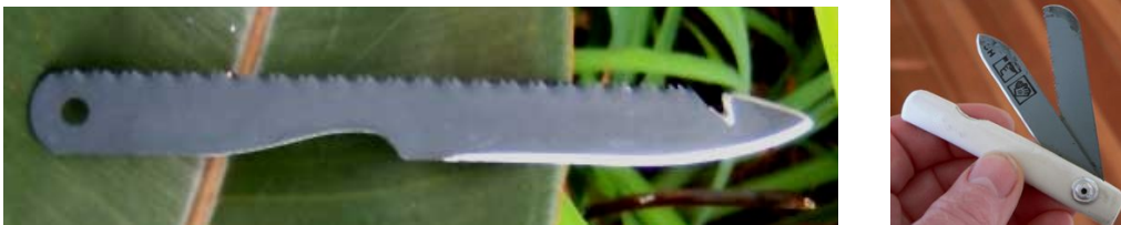
Broken hacksaw blades can be used to make tiny knives.
