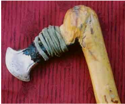
Simple axes, made from scrap steel or copper, and crooked tree limbs.
