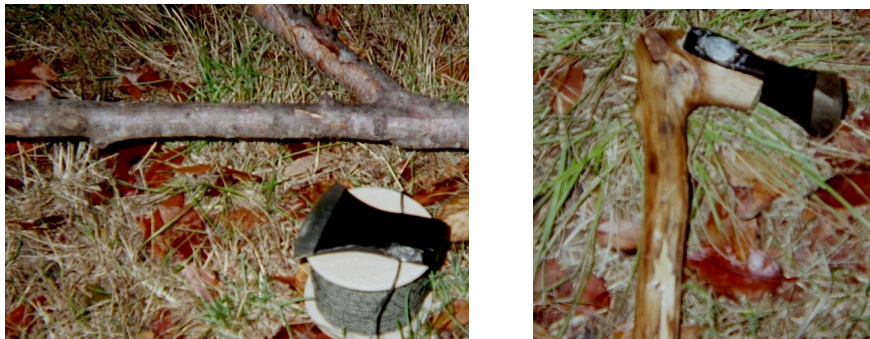
Selecting a forked branch for an adze handle, and making a notch for the axe head to fit into.
