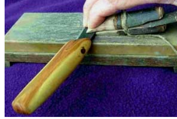
Improvised knife sharpening jig, being used to hone a scrap steel knife.
