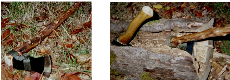
The completed improvised adze, showing the lashings, and using the adze and an axe to remove rotted wood from an open hollow log. (This log will be used, with the open side down, to make the entrance tunnel for a Den Trap).
