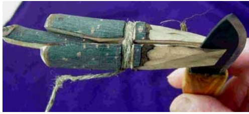
Improvised knife sharpening jig, being used to hone a scrap steel knife.
