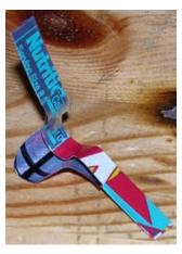
Padlock shims are one way to open a padlock without the key (they are used in pairs), and they can also be improvised from empty soda cans, or beer cans, like the example on the right.
