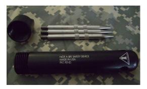
Grappling Hooks: These miniature grappling hooks disassemble, and store in the handle.
