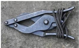
Wire Cutters: Used for defeating barbed wire obstacles, and for constructing them.
