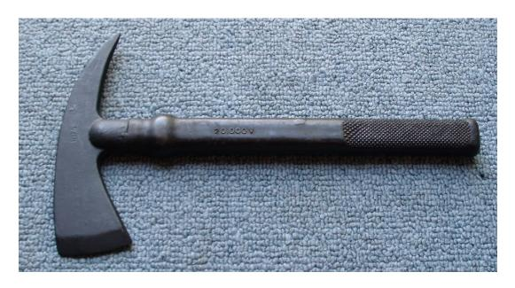
Crash Axes: Crash axes are used to cut your way out of a downed aircraft, but they will chop and pry through most barriers. Surplus units have insulated handles, for cutting through power lines.
