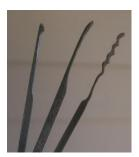
Here is a wire snap pick, with a rubber band spring, and picks made from hacksaw blades.
