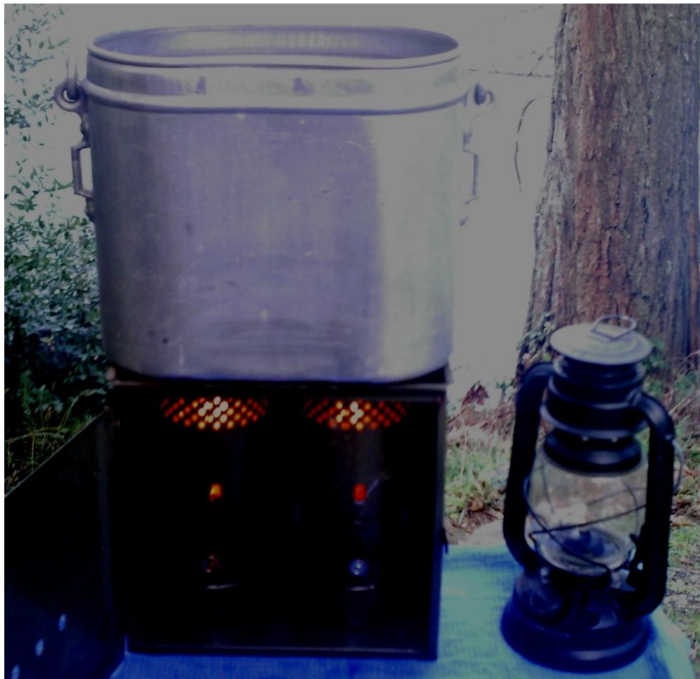
Two heaters can boil several gallons of water, while the metal box supports the weight of the pot.
