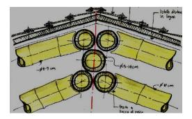
Bamboo "I-Beam", design, for roof beams, bridges, and other load-bearing applications.
