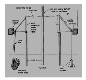
Bamboo water wheel (used to drive a remote well pump).
