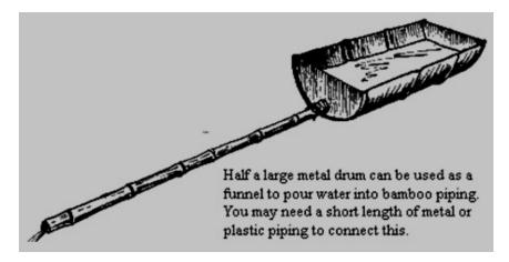
Bamboo pipes, with drum starter funnel.
