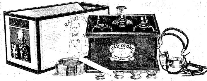
FIG. 49.—The "Radiofone." A loose-coupled type of receiver with stud-switch tuning for aerial inductance, stud-switch inductance-tuning in secondary circuit and variable condenser across latter for fine tuning. Enclosed "permanent" type detector.
