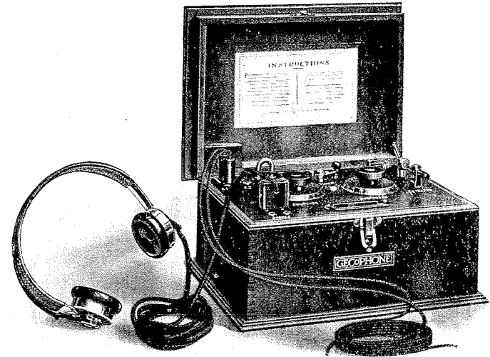
FIG. 48.—The Gecophone Crystal Set No. 2. A receiver of the loose-coupled type. The aerial circuit is tuned with a tapped switch and the detector circuit with a condenser. The coupling between the two circuits is adjusted by means of a coil which rotates within another. One of the few receivers in which a testing buzzer is incorporated.
