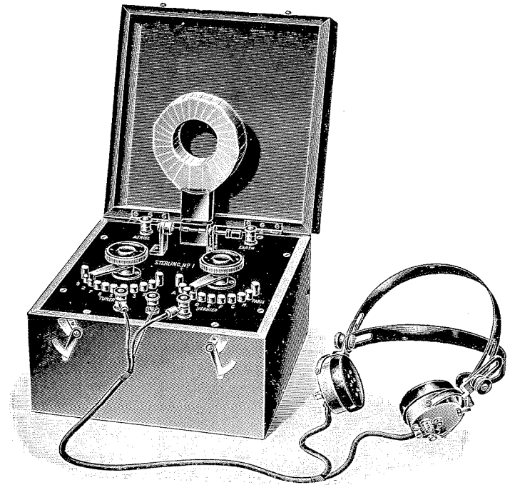
FIG. 23.—The Sterling No. 1 Crystal Receiver. The circuit is that of Fig. 21, with addition of the demountable coil for Eiffel Tower signals.
