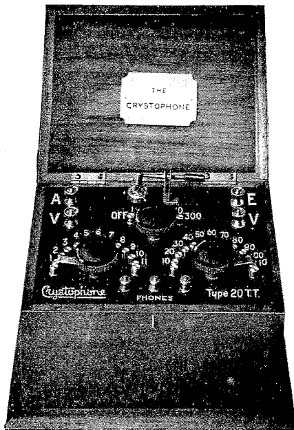
FIG. 24.—Crystophone Receiver with Stud Switches. The circuit is similar to Fig. 21, but a switch in the centre adds further inductance in large steps. The terminals V are used when a valve is added.
