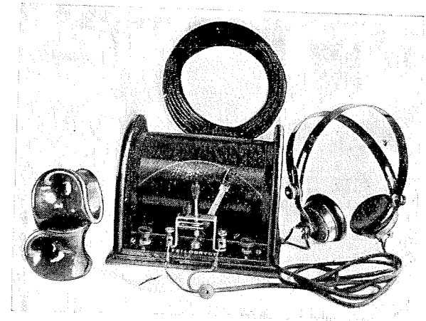
FIG. 20.—Simple Crystal Receiver utilising the Circuit of Fig. 11, and the Slider Method of Fig. 18. A coil of aerial wire is shown in the background and aerial insulators on the left.
