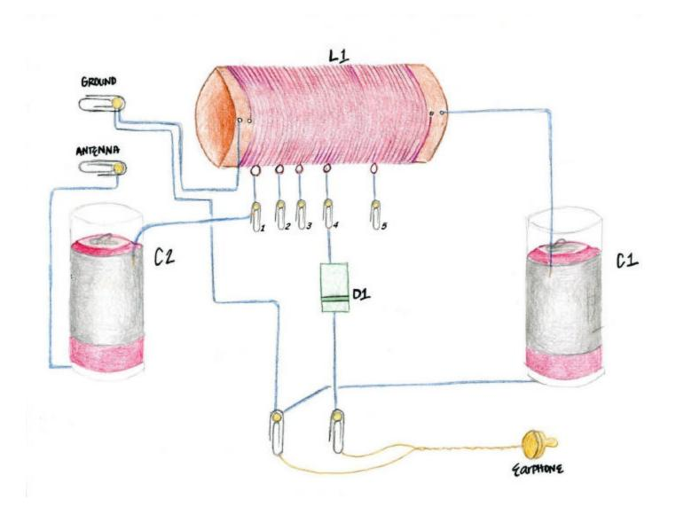
The above is a pictorial diagram of the crystal radio to show the approximate physical placement of the components.
