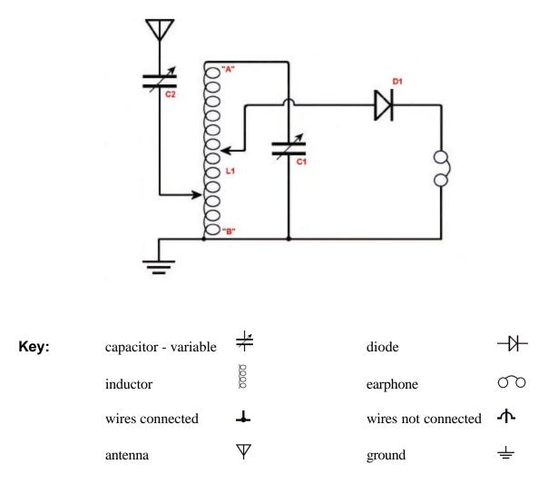
The above schematic diagram shows the electrical wiring of the crystal radio. Schematic diagrams are used by persons involved in the assembly and/or trouble shooting of electronic devices. The arrow on the coil represents an adjustable connection to the coil.
