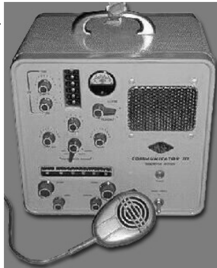
The classic Gonset Communicator, aka “Gooney Box”. Available in six and two meter band versions. A popular Cold War-era Civil Defense radio.
