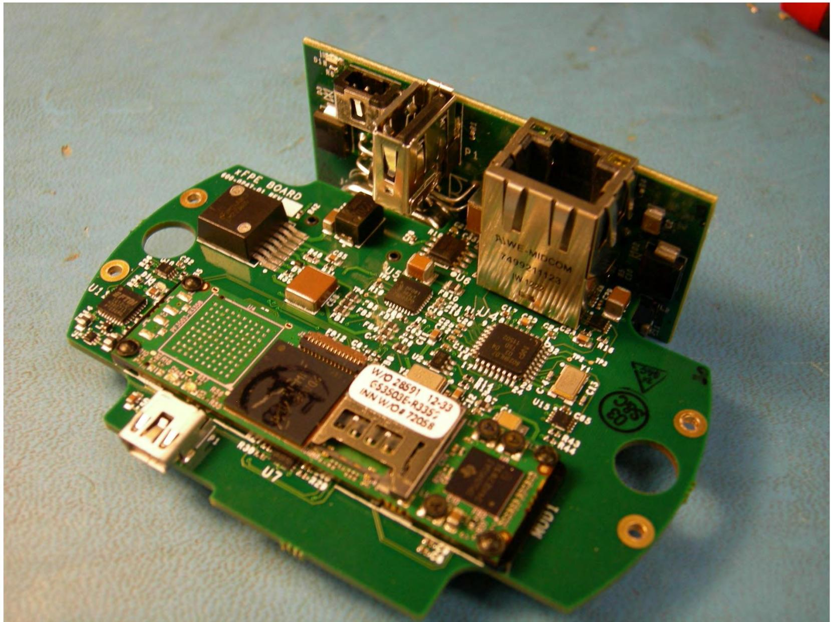
Radio microcontroller and SAM (Security Access module)
