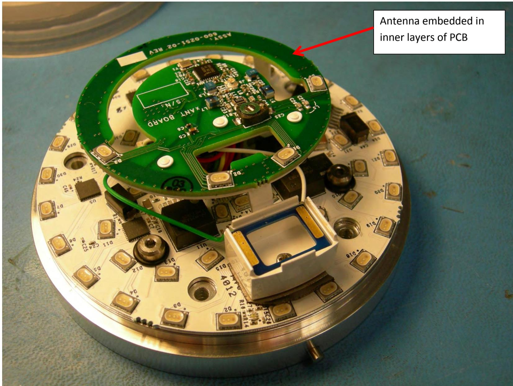
Antenna embedded in inner layers of PCB
