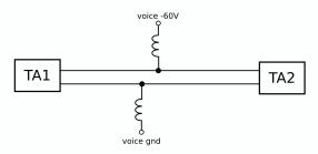
Coils are actually part of a relay. A special telephone relay with two coils and a single anchor can be used, but for now, it's okay to use two separate 24V relays. T coils pass direct current to power the phones, but resist alternating voice current and force it to go through another phone, rather than back through the power supply.
