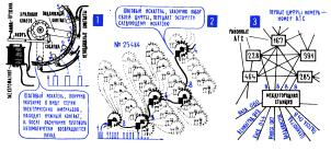
This mechanism can count pulses coming from a phone and advances its moving contacts to the next position. Most stepping switches are unable to step backward; when reset is needed, they continue to step in full circle until they get home.
