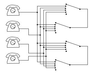
Switch operation may be driven by pulses coming from the phone, which is slow, or it may be free switching, where the switch quickly steps itself until it finds the right position.
