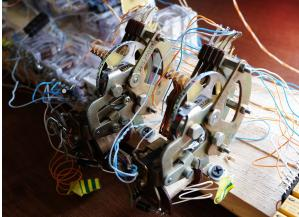
As well as a Tesla FN 935. Tesla was an electronic components manufacturer in Czechoslovakia, which made fine audio amplifiers and other audio equipment. It also developed special hardware for military use, including phone-line multiplexers, transmitters, and this 6-plane, 12-pole stepping switch.
