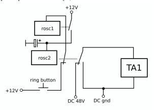
A phone handset shouldn't be lifted during the ring cycle, as the voice circuit on newer phones can be damaged by the ring current. I blew up one of my phones this way. Also, direct voltage must be mixed with alternating voltage, it is required for some phones to operate correctly.
