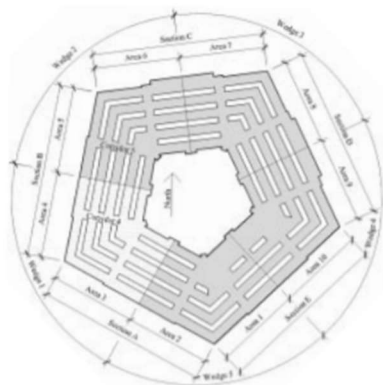
Figure 2.3 Designation of areas and sections used in the original construction and of wedges used in the ongoing renovation; Wedge 1 is hatched.
