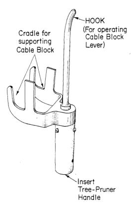
Fig. 5-D Cable Block Lifter
