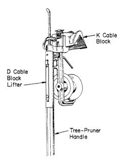
Fig. 6-D Cable Block Lifter (With K Cable Block)
