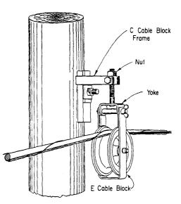
Fig. 9—C Cable Block Frame (With E Cable Block Installed)
