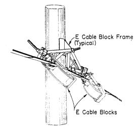
Fig. 10—D Cable Block Frame (With E Cable Block Installed)
