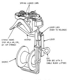
Fig. 3—K Cable Block
