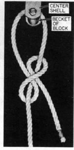
Fig. 17—Tying a Block Becket Bend
