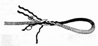
D-AFTER COMPLETING FOUR TUCKS, ROLL SPLICE BETWEEN TWO FLAT SURFACES AND TRIM SURPLUS ENDS. \*
