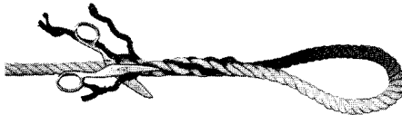
E- AFTER COMPLETING TWO HALF TUCKS, ROLL SPLICE BETWEEN TWO FLAT SURFACES AND TRIM SURPLUS ENDS.*
