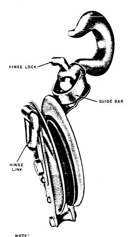
HOOK TILTED ASIDE FOR PLACING OR REMOVING WIRE ROPE WINCH LINE.
