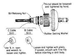
Fig. 4 - Replacing Bit for B and C Cable Drills
