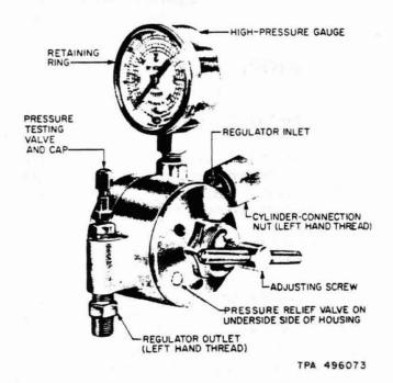
Fig. 1—B Pressure Testing Regulator
