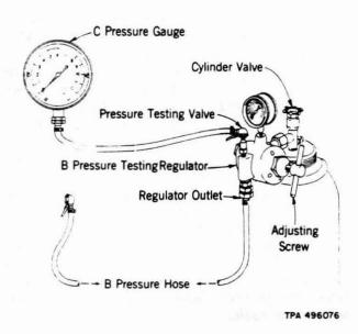
Fig. 6—Testing B Pressure Testing Regulator
