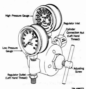
Fig. 3—C Pressure Testing Regulator
