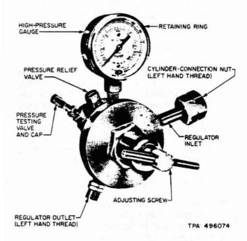
Fig. 2—B Pressure Testing Regulator—Alternate Design
