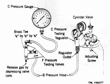
Fig. 7—Testing C Pressure Testing Regulator
