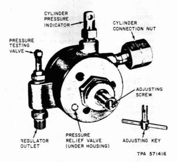
Fig. 4—D Pressure Testing Regulator
