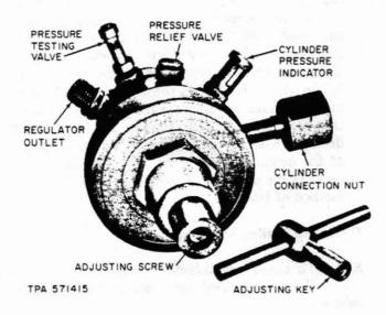
Fig. 5—D Pressure Testing Regulator—Alternate Design
