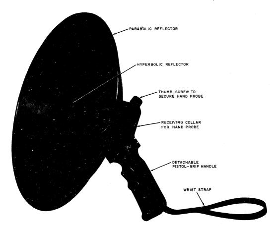
Fig. 14-B Ultrasonic Reflector
