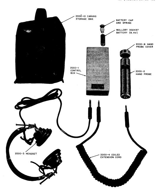
Fig. 12—Malor Group A ULT 2000 Ultrasonic Leak Locator
