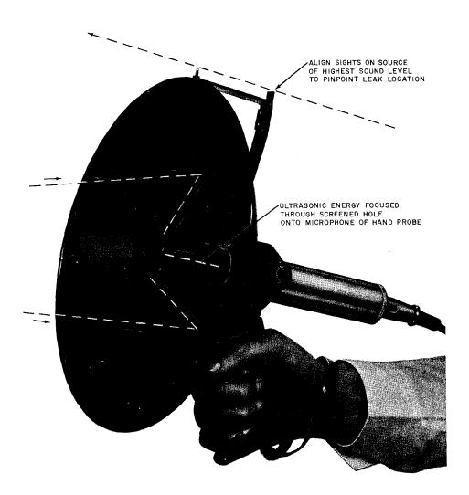
Fig. 15—B Ultrasonic Reflector—Principle of Operation
