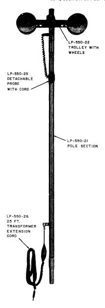
Fig. 7-Lumidor LP-560 Overhead Trolley
