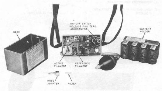
Fig. 2-E Gas Indicator Disassembled
