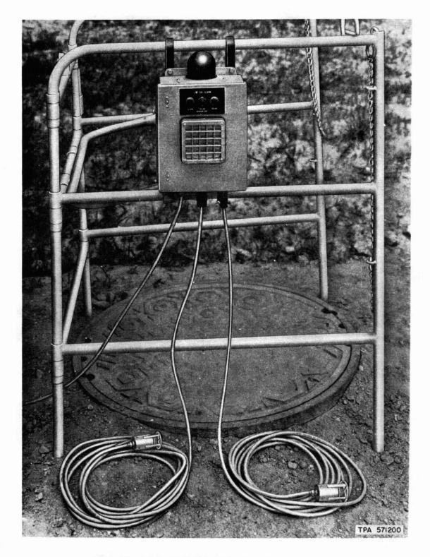
Fig. 3—Gas Monitor Attached to Outside of Manhole Guard
