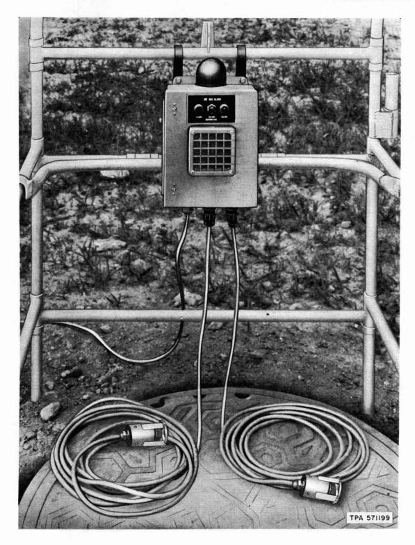
Fig. 2—Gas Monitor Attached to Inside of Manhole Guard
