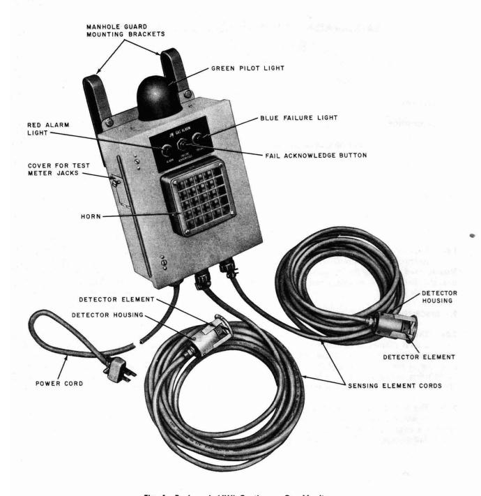
Fig. 1—Bacharach (JW) Continuous Gas Monitor
