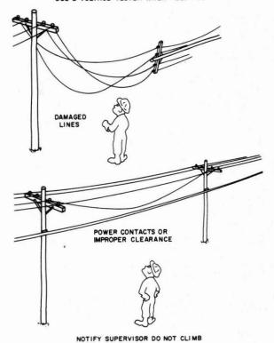
Fig. 6—Visual Inspection for Potential Electrical Hazards
