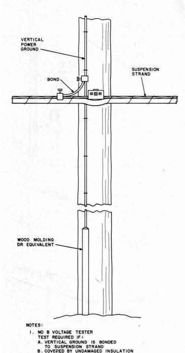
Fig. 7—Vertical Power Ground—Conditions Not Requiring Use of B-Voltage Tester
