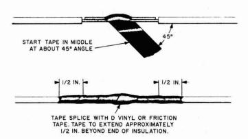
Fig. 5—Repairing Broken Cord
