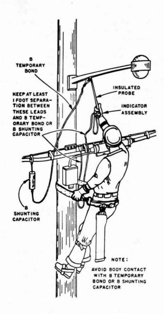
Fig. 12—Use of B-Shunting Capacitor
