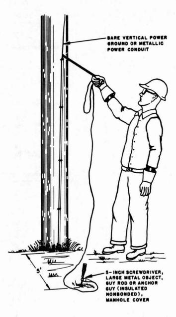
Fig. 10—Testing Vertical Power Ground
