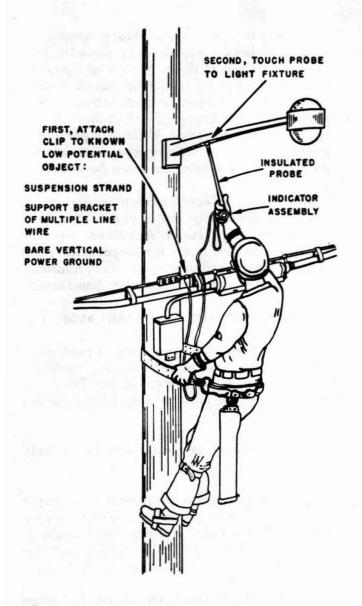
Fig. 11—Testing Street Light Fixture
