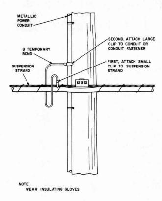
Fig. 13—B-Temporary Bond Attachment to Metallic Power Conduit
