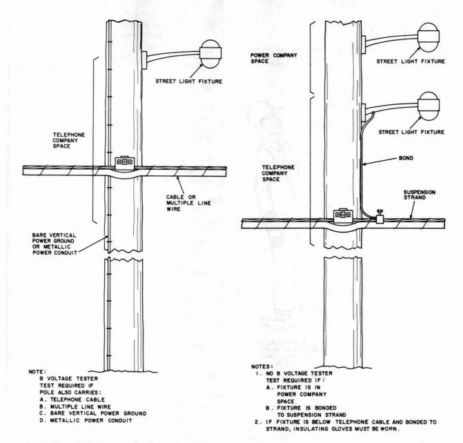
Fig. 8—Street Light Fixture—Conditions Requiring Use of B-Voltage Tester
