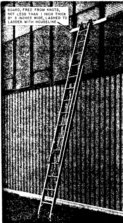
Fig. 38—Ladder Placed in Front of Window
