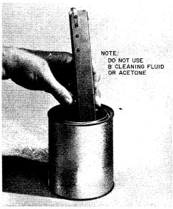
Fig. 8—Soaking F Connector Presser
