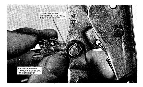
Fig. 4—Removing Sidewall to Open Through Slot
