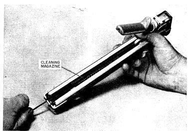
Fig. 9—Cleaning F Connector Presser With Brush
