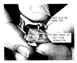
Fig. 2—Contacting Joint—IMPORTANT—Reseal per 2.01(b)(3)
