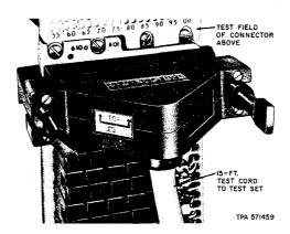
Fig. 4—Front Tap Shoe Mounted on Connector Test
