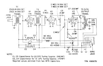
Fig. 2—99B Test Set—Circuit Diagram
