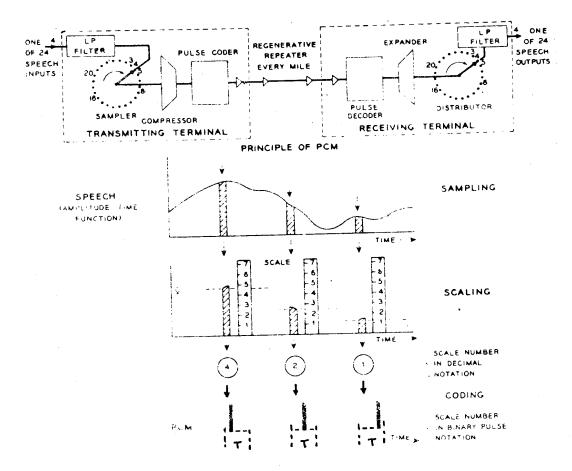
Figure 16-6 Pulse Code Modulation
