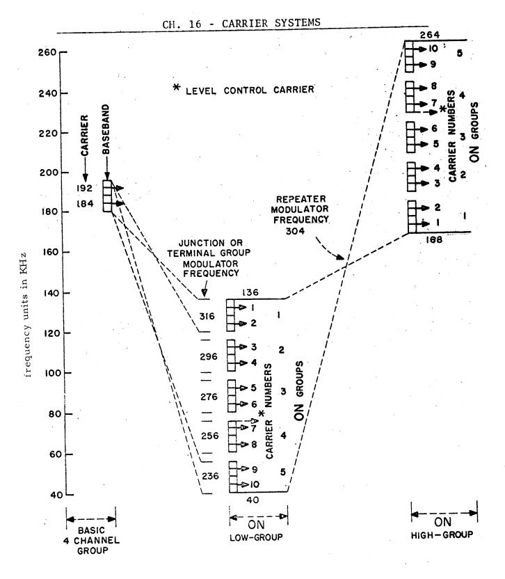
Figure 16-22 ON1 Carrier System Modulation Plan
