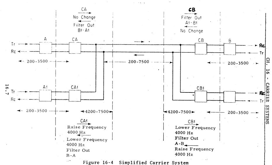
sufficient. This range will allow one subscriber to identify any other subscriber. The carrier frequencies are steady frequencies other than voice frequencies, usually higher than the voice range. Superimposing is accomplished by modulation.
