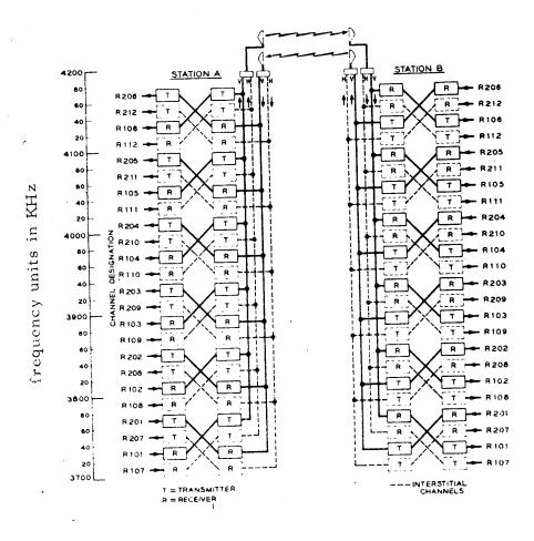
Figure 16-28 Frequency Plan for 12 Channels
