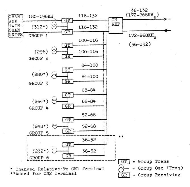
Figure 16-23 Block Diagram of 24 Channel ON2 Terminal
