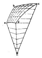
Figure 16-29 Delay Lens Antenna
