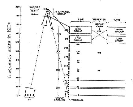
Figure 16-21 Type O Modulation Plan
