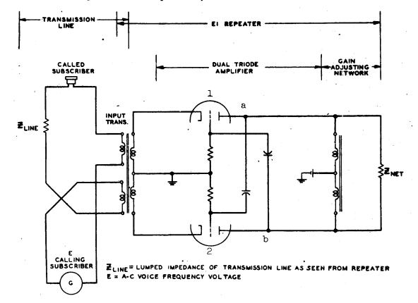
Figure 17-8 Simplfied Schematic of El Repeater
