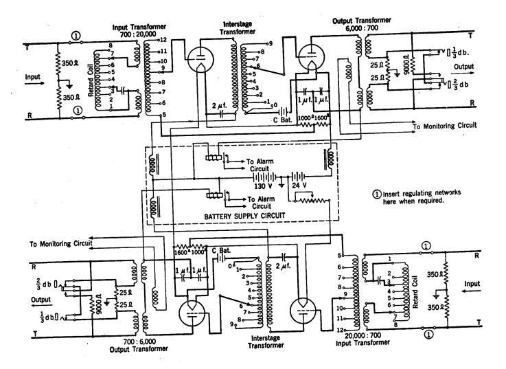
Figure 17.2 44-Type Telephone Repeater Circuit
