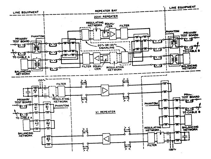
Figure 17-3 (above) - Block Schematic of an Intermediate 22A1 Repeater; (below) - Block Schematic of a V1 Repeater.
