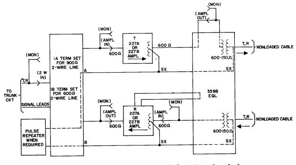
(B) 24V4 Repeater Arranged for Non-Loaded Cable Requiring Gain and Loop Signaling
