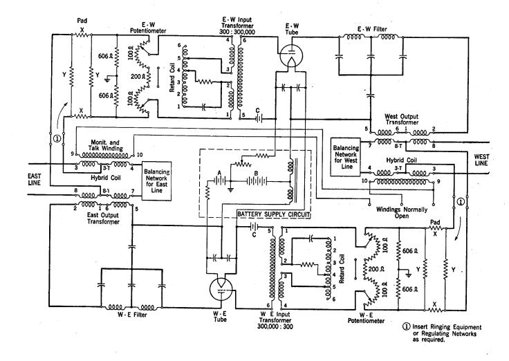
Figure 17.1 22-Type Telephone Repeater Circuit
