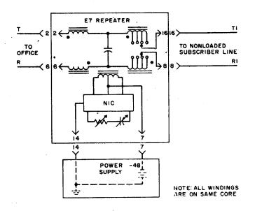
Figure 17-12 Simplified Schematic of E7 Repeater
