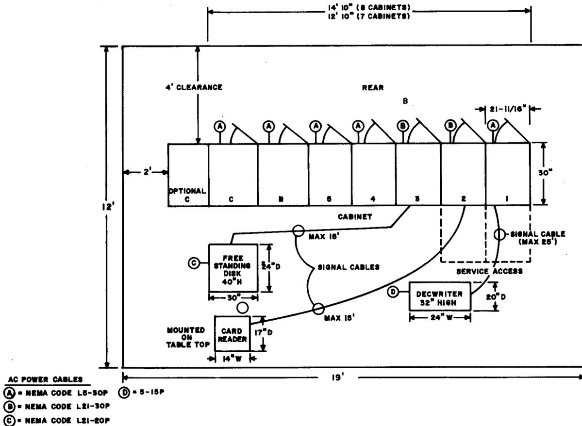
Fig. 4—EADAS/NM CCU Sample Floor Plan
