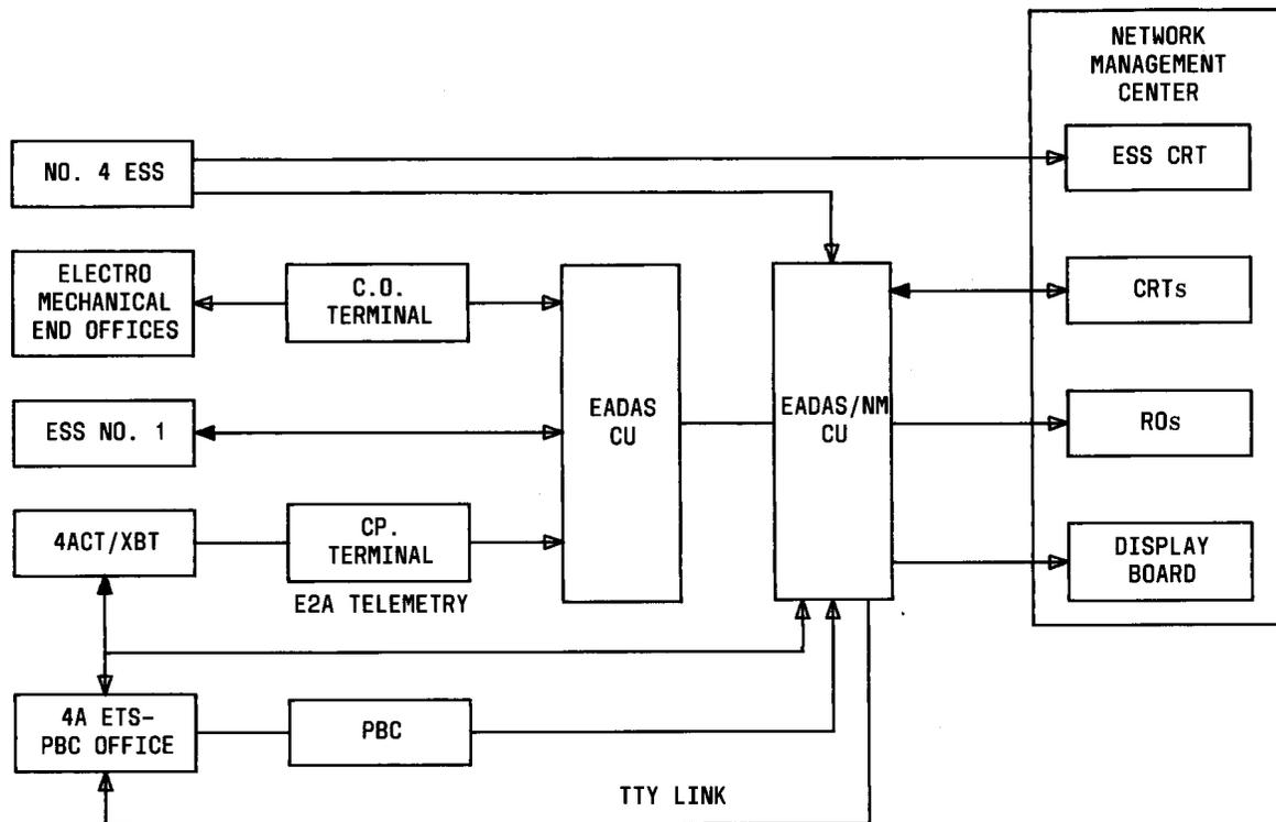
Fig. 1—EADAS/NM Generalized Arrangements
