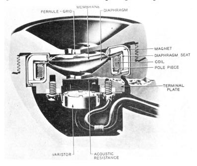
Figure 2-7 Ring-Armature Receiver
