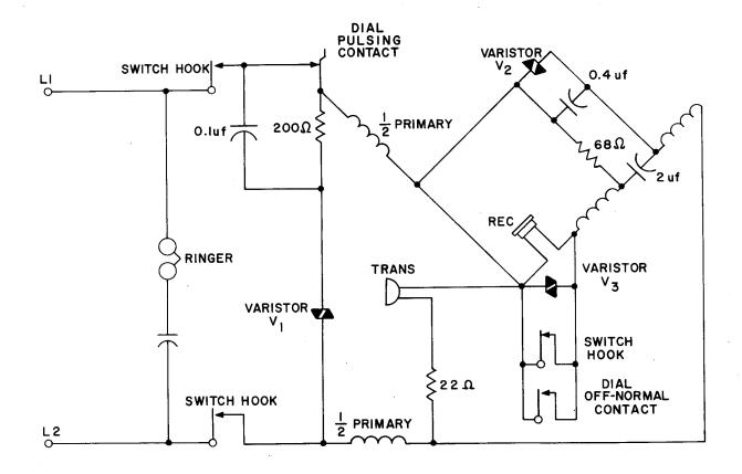
FIGURE 2-13 - Complete Circuit of Type 500D Telephone Set
