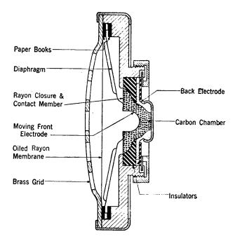
Figure 2-4 Cross-Section of Transmitter Unit
