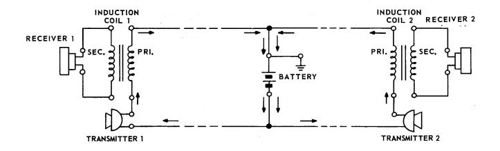
Figure 2-9 Common Battery Telephone System
