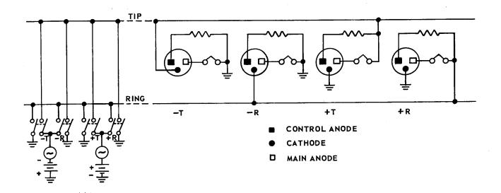
Figure 2-22 4-Party Selective Ringing Using 3-Element Cold-Cathode Tubes
