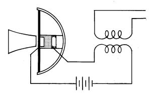
Figure 2-3 Principle of the Telephone Transmitter
