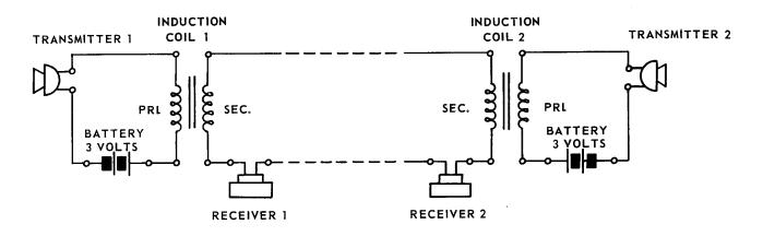
Figure 2-8 Local Battery Telephone Circuit
