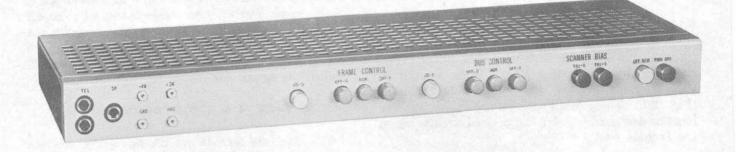
Fig. 14—Scanner Control Panel Using Type 1 through 5 Ferrods
