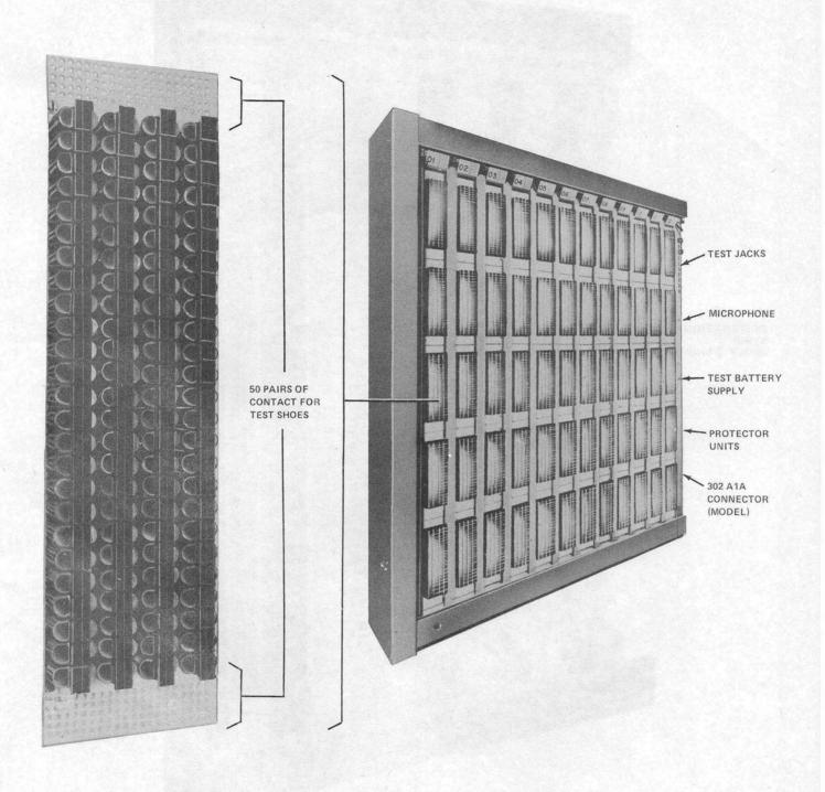
Fig. 2—Protector Frame, Front View
