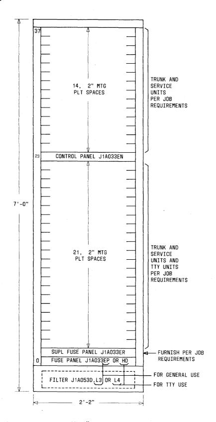
Fig. 5-Miscellaneous Trunk Frame
