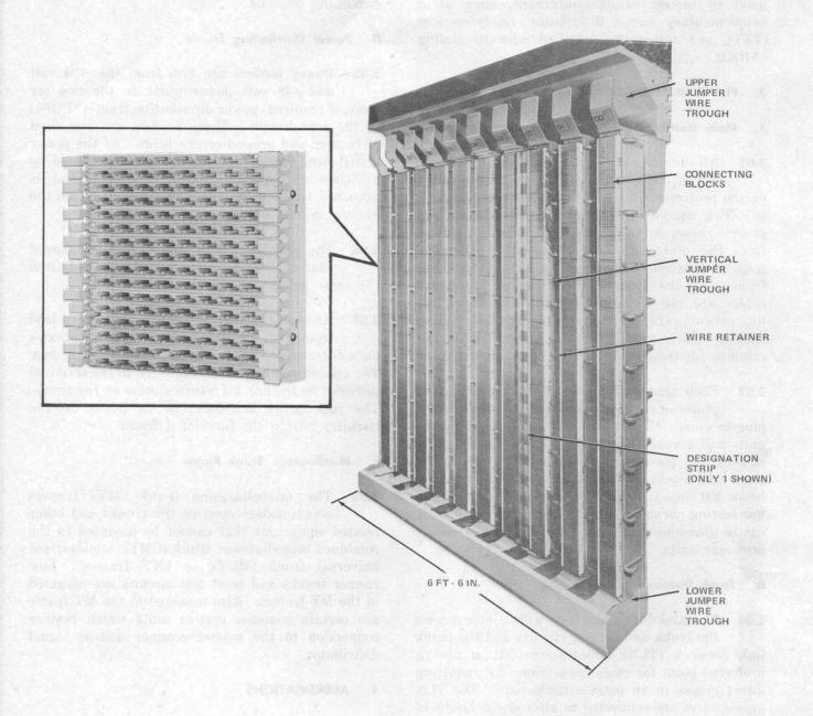
Fig. 1—Main Distributing Frame Module
