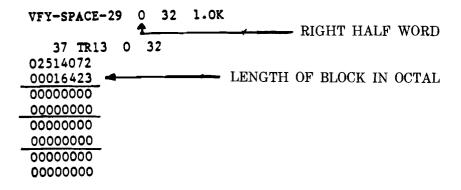
Figure 14 - Right Half (32 or Greater) Length of Block Output Message TR13 (5.09, 5.10)
